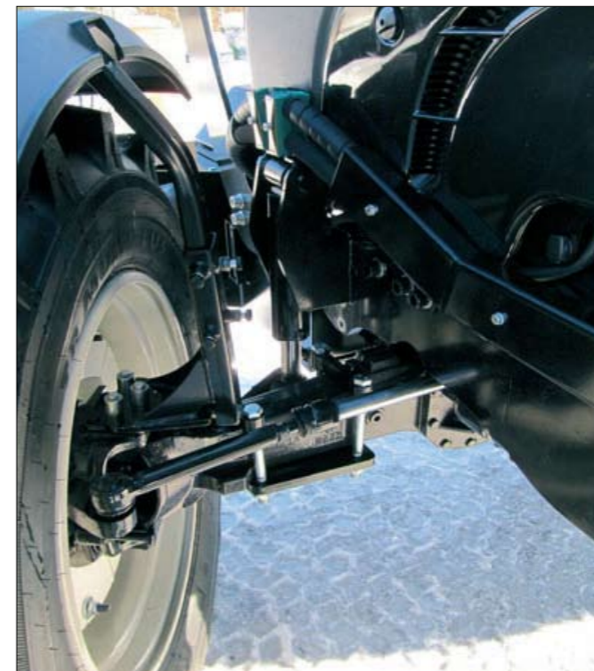
Front axle locking unit set for Valtra tractors without air-suspended axle. Set consists of two cylinders, hoses and valve.
