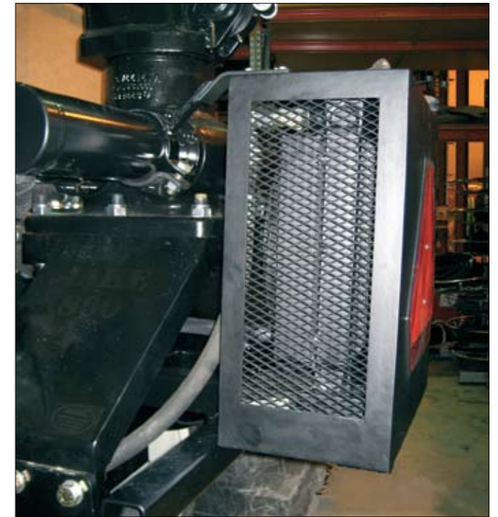
Oil cooler. In warm conditions, operating a harvester head or a felling grapple, is an oil cooler needed
