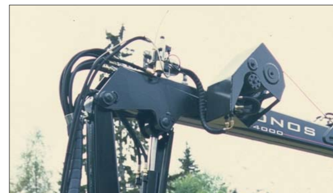
Radio controlled hydr.winch. 1400 kp, wire: Ø 6 mm, length 35 m
