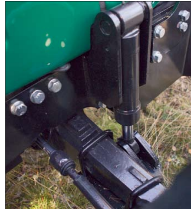
Front axle locking unit set for Valtra tractors without air-suspended axle. Set consists of two cylinders, hoses and valve.
