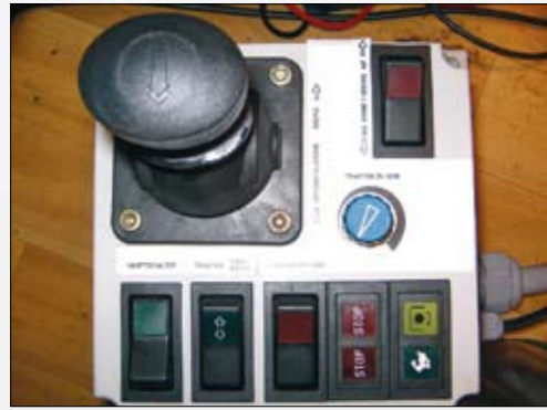
Control unit for trailer (in tractor cabin)
