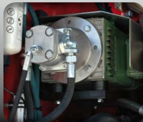
Generator for electromagnet driven by a hydraulic motor and mounted on silent blocks
