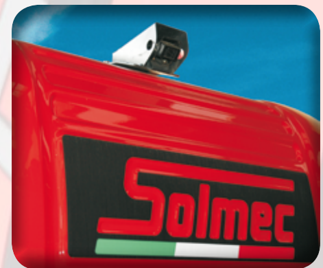
Rear camera on counterweight with 7" color display into the cabin. It's also possible to fit a camera on the secondary stick. (as option)
