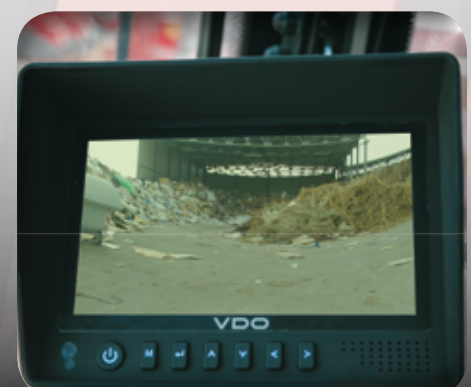
Rear camera on counterweight with 7" color display into the cabin. It's also possible to fit a camera on the secondary stick. (as option)
