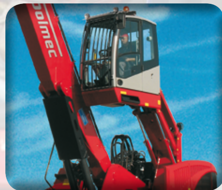
Operators cabin with hydraulic parallelogram elevation has a 5,2 m high reach (operator's eye). It is possible, on request, to arrive to 6,0m high reach.
