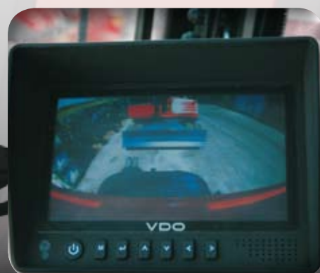
As option, rear camera on counterweight with 7" color display into the cabin. It's also possible to fit a camera on the secondary stick.
