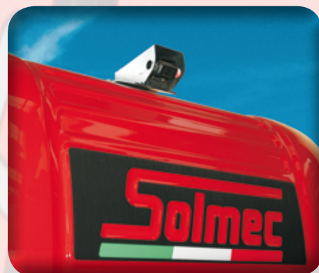
As option, rear camera on counterweight with 7" color display into the cabin. It's also possible to fit a camera on the secondary stick.
