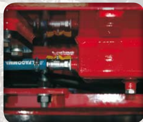
Safety taps on the diesel and oil tank for a quicker and easier maintenance of the machine
