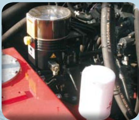
Centralized automatic greasing system (as standard), to make easier service operations. Oil tank pressurized with air filter.
