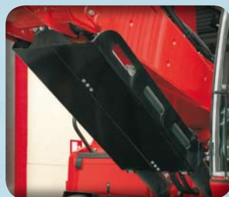
Hoist cylinder's rods protection available on request.
