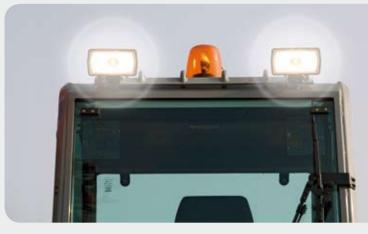
**Halogen working lights** and the orange flashing beacon fitted on the top of the cab guarantee a good visibility during the darker hours of the day. It is possible, as option, to fit extra working lights on stick and on the counterweight to increase visibility.
