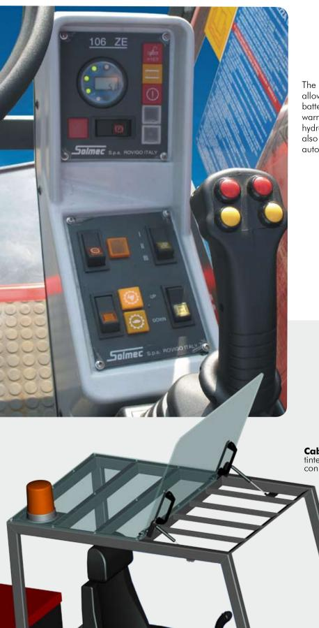
The clear visual instrumentation panel allows monitoring of all machines functions: battery charge level, electric motor diagnostic, warning light for low hydraulic oil level, congested hydraulic oil filter, and stability limit. There are also controls dedicated to electric motor speed, automatic switch off, parking brake, gear box.
