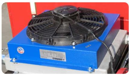
**The cooling of the hydraulic oil** is ensured by a large wide mesh radiator that allows a better temperature exchange thus avoiding occlusion of the air passages when working in a dust or contaminated air environment. The radiator is fitted with an thermostatically controlled electric fan.
