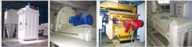
Coarse grinding + dust collecting Fine grinding Pelletizing Pellet grading
