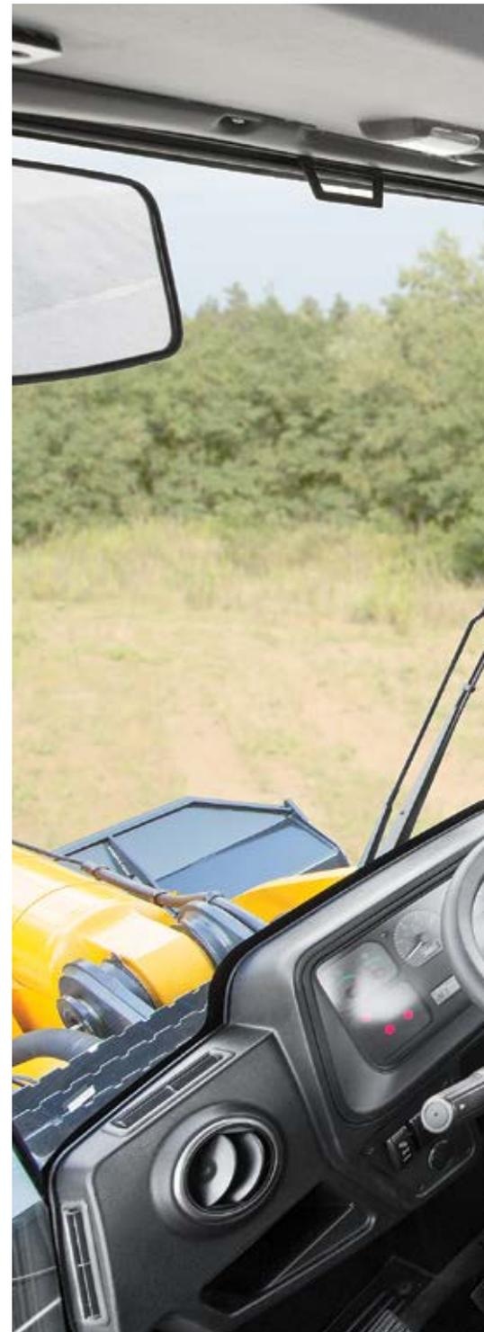
The cab protects the operator from noise and vibrations and is well ventilated. It has advanced climate control to handle the changing seasons and is completely sealed to prevent dust from entering the work place.
