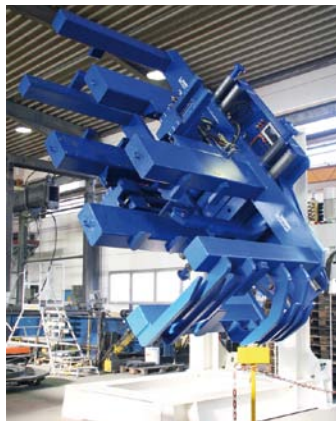
25T251W/099 – Inverter for steel sheets
