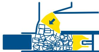
Prepress forces material into press chamber.
