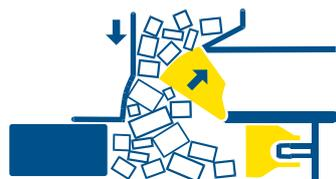
Prepress opens and material in hopper falls into press chamber.
