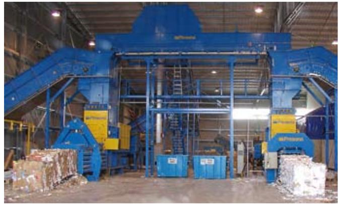
Two new balers were purchased for the plant, one LP 100 DH4S and one LP 140 XH2S with a feed opening of 1100 x 2250 mm. The LP 140 XH2S has a combined press force of 210 tons, a bale format of 1100 x 1100 mm and 2 x 75 kW electric motors. This giant presses everything from cardboard to shredded industrial waste and produces up to 50 tons or over 800 cubic meters per hour.
