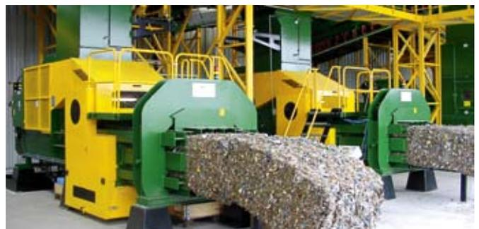
The material, which is delivered to incineration plants for energy production, must be baled for efficient handling, storage and transport.
