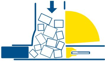
Prepress and main press in their starting positions. Press chamber full.
