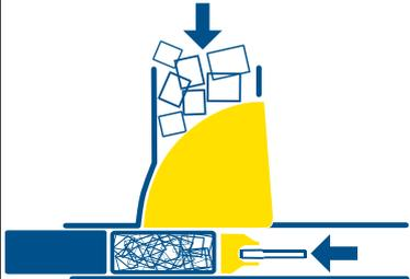
Main ram compresses material with maximum pressure. Conveyor continues to feed material to hopper.
