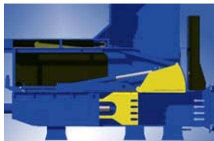
does not need to be cut off – which reduces both wear and the risk of stoppages. Here there is a pre-compression of the material and all of the power is used for compression
