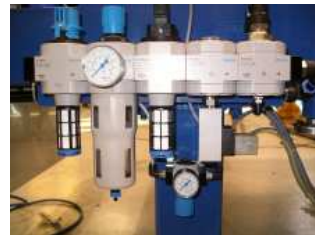
Details of the filtering system and pneumatic control
